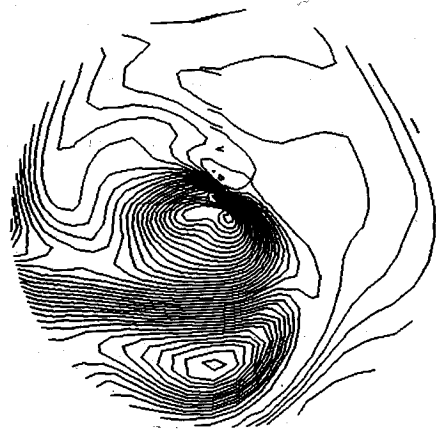
Fig. 10 Vorticity contours at the inlet duct exit.
